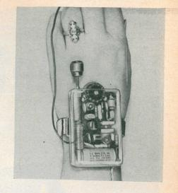
receivers. A GT760 acts as the detector and GT20 and GT81 transistors fill out the audio stages.
