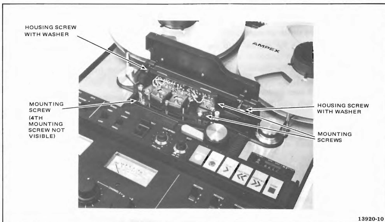
Figure 5-22. Head Assembly Removal
