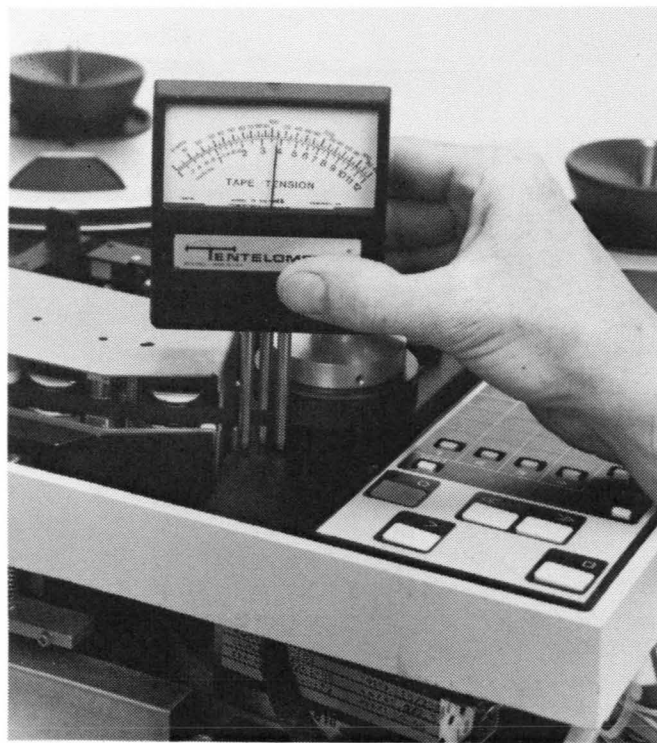
Figure 5-25. Measuring Tape Tension
